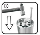
Tap on side of footvalve to twist it in a vertical position.
